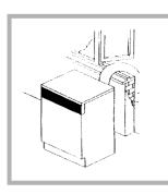
1. The end of the tube should be directed downwards, to prevent warm moist air from condensing in the room or in the dryer.
